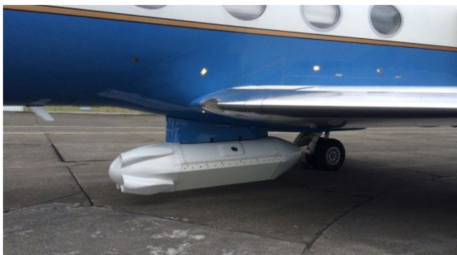
The polarimetric L-band SAR instrument on NASA's aircraft at Sola, Stavanger in June 2015. Photo: Camilla Brekke, UiT.
