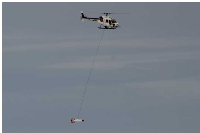
Electromagnetic systems for ice thickness measurements. EM31 in sledge (left) and EM-bird underneath the helicopter (right).
