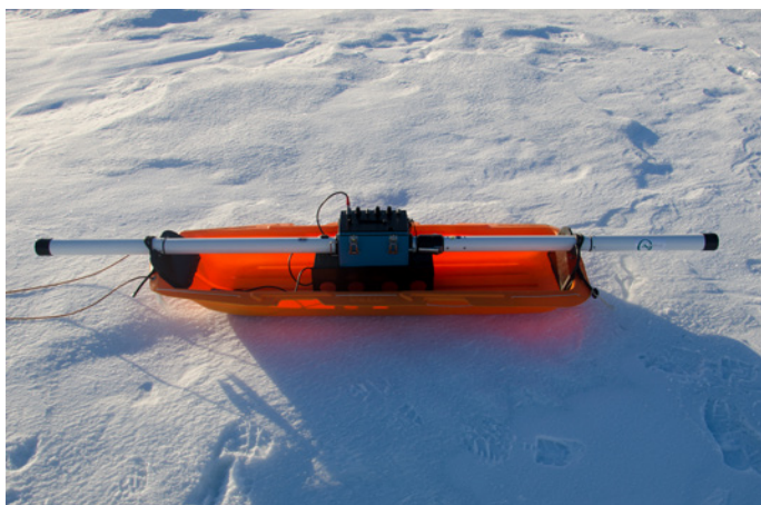
Electromagnetic systems for ice thickness measurements. EM31 in sledge (left) and EM-bird underneath the helicopter (right).
